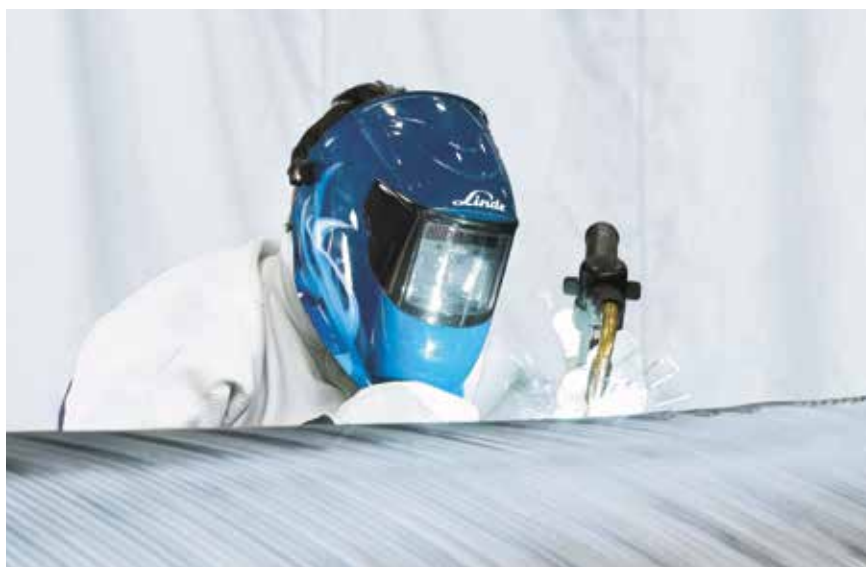
METAL INERT GAS WELDING ON AN ALUMINIUM PIPE.
